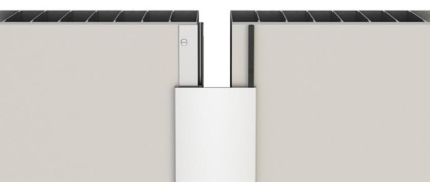
This surface-mounted metal wall and ceiling cover is designed for interior applications where low maintenance or tamperresistant applications are desired. The free-floating aluminum center plate spans the joint and slides over the surface of the wall or ceiling to allow movement when required. The cover can be painted to match nearly any finish and is available in multiple metal finishes.
