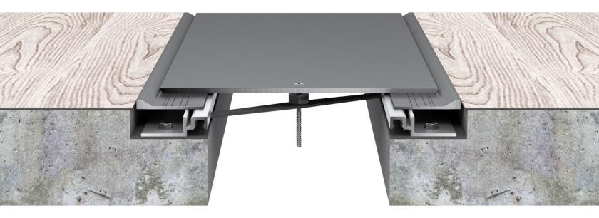
This surface-mounted or flush-mounted metal floor cover is for interior or exterior applications. The self-centering aluminum center plate allows for thermal and seismic movement. Cover offers a variety of aesthetic and performance variations, depending on model.
